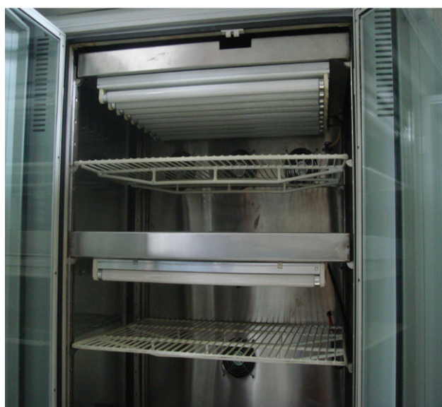
Fig. 1. Schematic experimental device and chamber photo for photodegradation of PAHs on soil surfaces.
